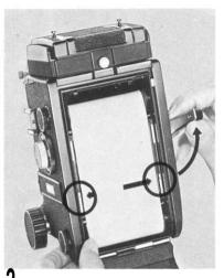
Pull out the leader paper of the film and guide it into the slit of the take-up spool, turn the film wind crank (6) clockwise until the start mark on the leader paper matches the start marks (39) on the camera.
