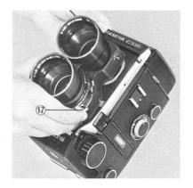
To attach another lens to the camera body, carefully position the lens so that the lens shutter cocking lever (17) connects with the cocking lever on the camera body. This operation is correctly performed by previously cocking the lens shutter with the fingers, first inserting the lens from the cocking lever side on the body. Clamp the lens catch (20) to its original position, and turn the lens change knob (24) clockwise to the "LOCK" position. With this operation, lens replacement is completed.
