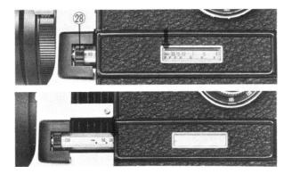
A distance scale is provided on the left side (viewing the camera held for photographing). By turning the knob (28), set the distance scale to coincide with the lens used, so that the scale faces horizontally.
