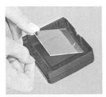
When using a 55mm or 65mm lens, set the dial (25) to 80 and attach the parallax correction plate for 55mm/65mm lenses to the focusing hood.
