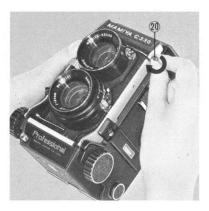
Tip the camera so that the lens faces upward. and while firmly grasping the lens barrel pinch the head of the lens catch bracket (20), press the head toward the camera body, push it down to release the lens catch, and remove the lens.
