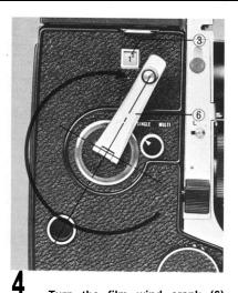
Turn the film wind crank (6) clockwise until it stops. Figure 1 appears on the exposure counter (3) at the position where the crank stops diagonally upward, and the shutter is automatically set. Now the camera is prepared for the first exposure. The crank cannot be turned in reverse.
