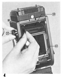
Open the back cover and pull out the spool change knob (22), then insert an empty spool into the takeup spool chamber (38) so that it engages the winding axis. Release the spool change knob.
