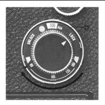
After changing a lens, set the parallax correcting dial (25) to the focal length value of the mounted lens. Regarding 55mm and 65mm lenses, set the parallax correcting dial to 80. then attach the parallax correction plate for 55mm/65mm lenses to the focusing hood. (Refer to p. 15 for handling method of the focusing hood).
